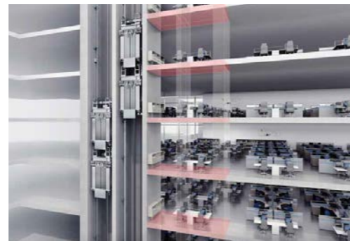
Rentable space with double-deck elevators
